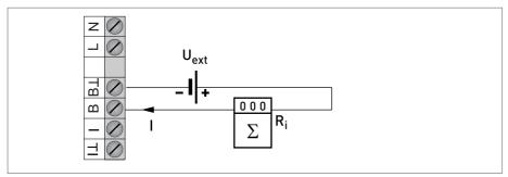
Figure 4-14: Pulse output (passive) for Ex-i Modis
