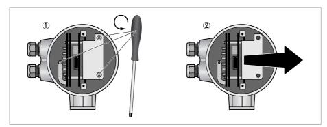
Figure 7-4: Removing electronics unit
