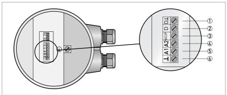
Figure 4-4: Terminals for instrument with Profibus PA (non Ex).
