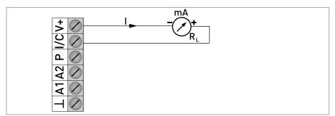
Figure 4-10: Current output (active)
