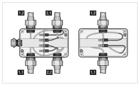
Figure 4-1: Connection of the sensor cables for dual beam (left) and single beam (right) building construction (sensor side)
