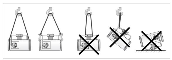
Figure 3-1: Correct lifting with the help of straps or crane hooks.
