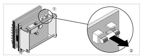
Figure 7-5: Removing fuse
