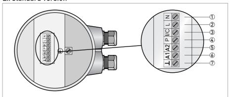
Figure 4-6: Terminals for Ex standard instrument
