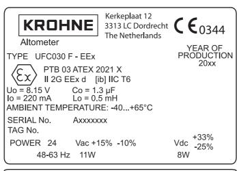
DO NOT OPEN ENCLOSURE WHEN ENERGIZED! WAITING TIME BEFORE OPENING OF THE FLAMEPROOF ENCLOSURE. T6 ≥ 20 MIN; T5 ≥ 11 MIN.
