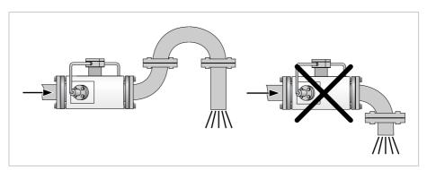
Figure 3-6: Ensure you have a completely filled pipe.
