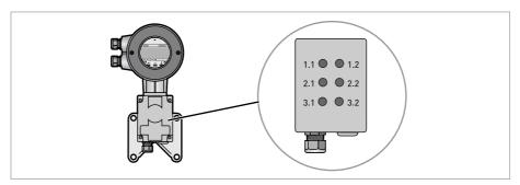
Figure 4-2: Connection of the sensor cables, converter side
