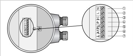
Figure 4-7: Terminals for Ex instrument with NAMUR
