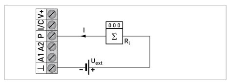
Figure 4-13: Pulse output (passive)
