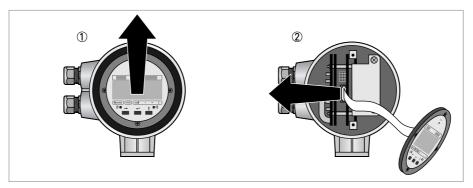
Figure 7-3: Disconnecting display cable
