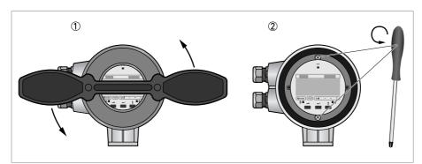
Figure 7-2: Removing display print
