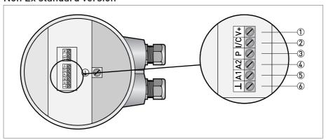
Figure 4-3: Terminals for standard instrument.
