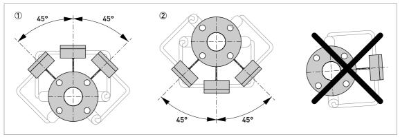
Figure 3-3: Allowed position of the flow sensor (up and down)
