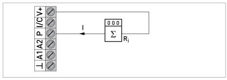
Figure 4-12: Pulse output (active)
