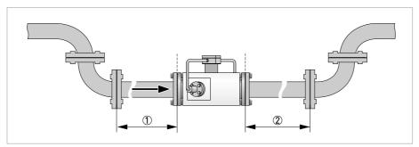
Figure 3-2: Recommended straight inlet and outlet
