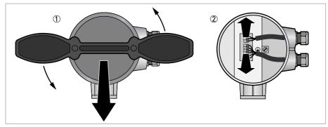
Figure 7-1: Switching off power
