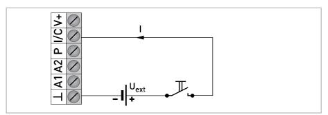
Figure 4-16: Digital input (passive)
