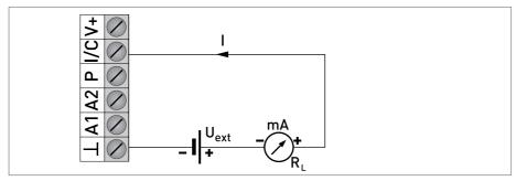
Figure 4-11: Current output (passive)
