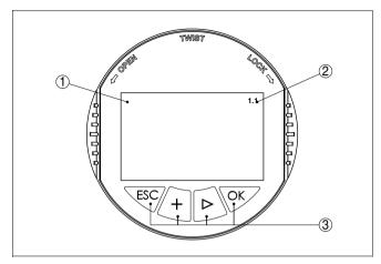
Fig. 21: Indicating and adjustment elements
