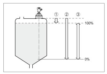
Fig. 4: Measuring range (operating range) and max. measuring distance
