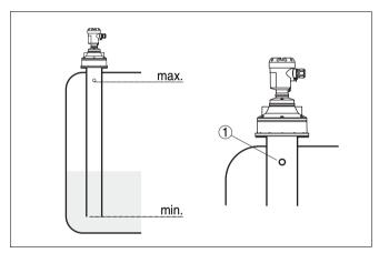
Fig. 14: Standpipe in a tank
