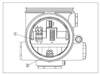
Fig. 18: Connection compartment, double chamber housing
