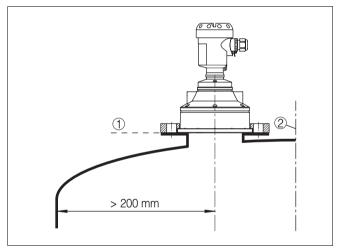
Fig. 5: Mounting on dished vessel tops
