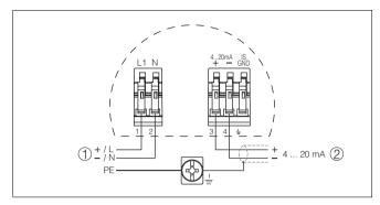
Fig. 19: Wiring plan, double chamber housing
