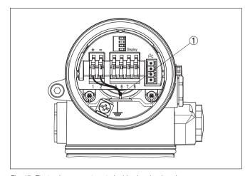
Fig. 17: Electronics compartment, double chamber housing
