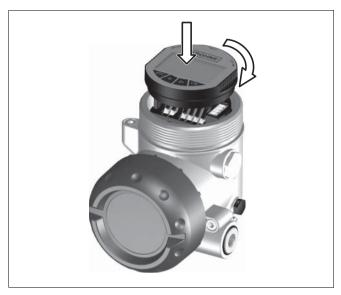
Fig. 20: Installation of the indicating/adjustment module
