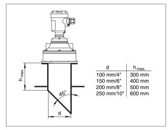
Fig. 7: Deviating socket dimensions
