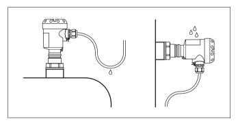
Fig. 2: Measures against moisture penetration
