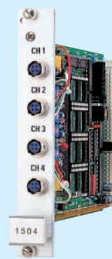
MODEL 1504 ●V module 4 ch (Air velocity)
