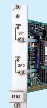
MODEL 1503* ●Pressure module 2 ch
