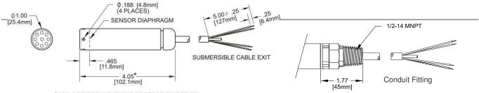
\*ADD 1.95" FOR LIGHTNING PROTECTION OPTION **Gland Cable Seal Configuration for ETFE Cable**
