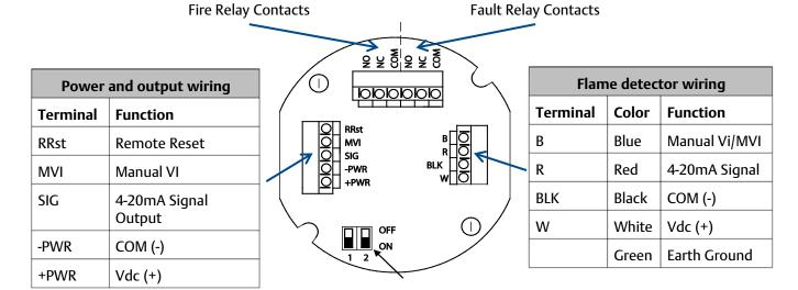
**Note:** Shield should be terminated at the Panel/PLC/DCS/RTU
