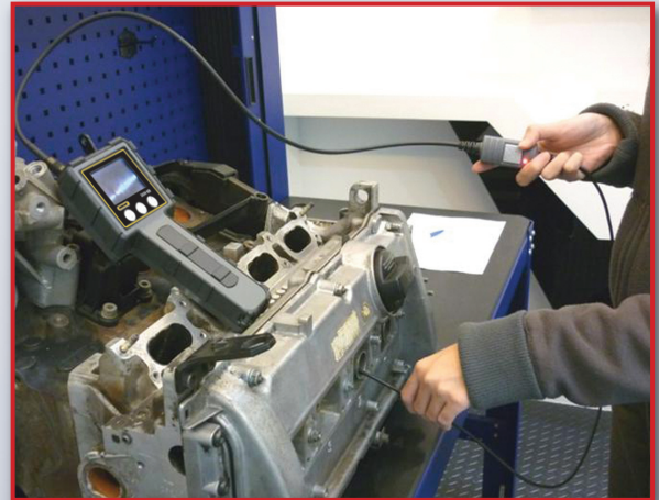
Inspecting the coolant passages of an engine block through the hole of a freeze/casting plug
