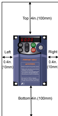
Figure 2.1 Mounting Direction and Required Clearances
