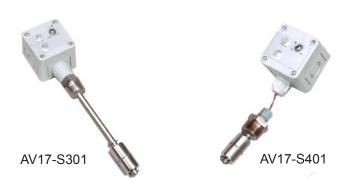
The general purpose, battery powered drum alarm provides reliable liquid level monitoring of 55-gallon drums. The stainless steel float assembly is available in three configurations including high alarm, low alarm or high and low level alarm. In the event of an alarm condition, the battery powered LED will actuate to alert the user. Select the compact alarm which is mounted on the float stem, or the remote alarm which is separated from the float stem with a 72" (1.82m) cable.
