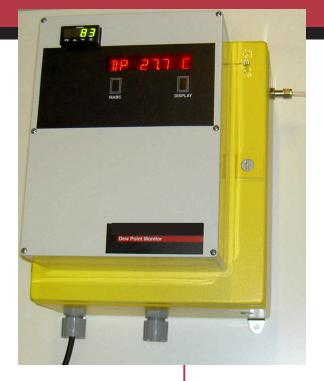
**DPS1** is a heated dew point hygrometer that can measure dew points up to 95 °C (203°F) and as low as -35 °C (-31°F). This integrated system includes a microprocessor based electronics, a chilled mirror dew point sensor, a sample flow meter/valve, a 3 foot heated sample line, assorted tubing and fittings all contained in a heated, temperature controlled NEMA-4 enclosure.
