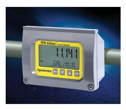
The Ultra is available in two versions: a stand-alone flow meter, and an energy flow meter used in conjunction with dual clamp-on RTDs. The energy flow meter measures energy usage in BTU, MBTU, MMBTU, Tons, kJ, kW, MW and is ideal for retrofit, hydronic and other HVAC applications.
