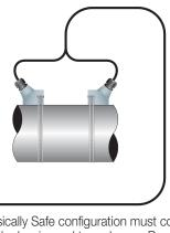
\* Intrinsically Safe configuration must contain both the barrier and transducers. Barrier must be within Class I Div. 2/Ex nA or General
