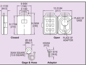
The **Model LPTK Gas Pressure Test Kit** is ideal for testing LP and natural gas lines and controls. The kit's gage shows if proper pressure is present or if a leak exists. The LPTK Gas Pressure Test Kit is available in two different gage ranges, and each gage is 3% full-scale accurate with an easy to use calibration screw on the back of the gage. It is easier to use than a manometer, and includes a sturdy case for added durability and safe handling.
