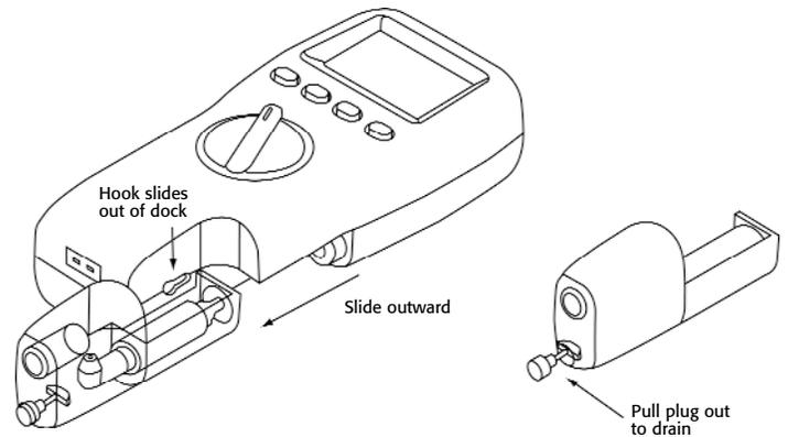
If condensate spills onto the skin or clothing, clean off immediately using fresh water, seek medical advice if problems occur. Ensure plug is replaced before performing combustion tests.
