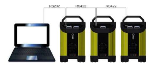
Note: The RS 422 standard specifies a maximum lead length of 1200M (4000ft). A true RS422 port will be required to realise such lead lengths. The Isotech conversion leads are suitable for maximum combined lead lengths of 10M that is adequate for most applications.
