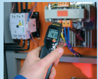
Measurement on live or moving parts
