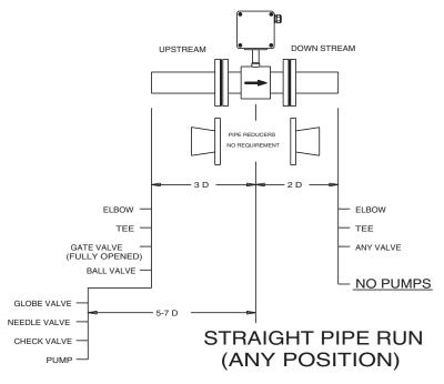
Figure 4: Pipe diameters
