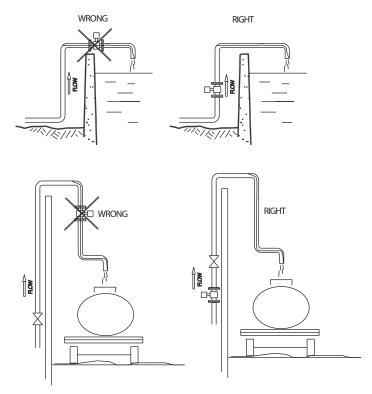
Figure 5: Proper installation locations
