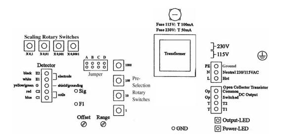
Figure 10: Rotary switch location
