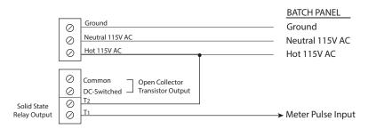
Figure 8: Connection for batch panels
