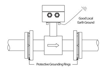
Figure 6: Protective grounding rings
