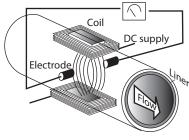
Figure 1: Meter operation
