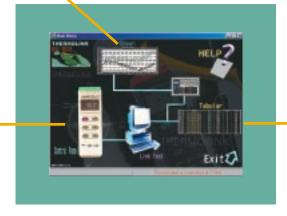
Clicking on the Auto Arrange section of the main screen opens the Control Panel, Realtime Graph, and Tabular windows, arranged in a non-overlapping display.
