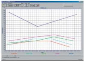
Easily see temperature trends and potential equipment problems by graphing data accumulated with the MX's data logging feature.
