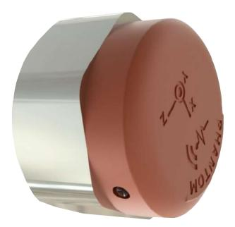
Use the symbol on the top of the Phantom to locate the axis in the right position.
