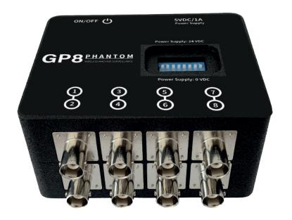
GP8 Can work with 5VDC power supply. Additionaly, GP8 works with Phantom Standar Gateway receiver, supporting more than 100 sensor at the same time.
